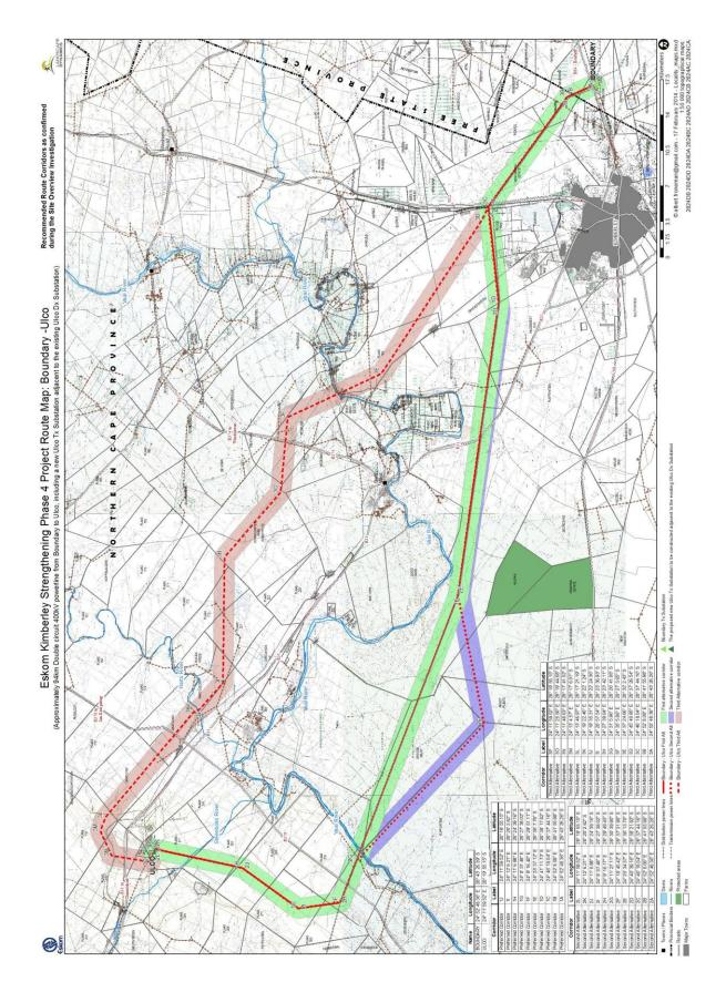
Figure 1: Map of proposed powerline route between Ulco and Boundary (Northern Cape), provided by Landscape Dynamics and Eskom.
